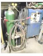
**Miller mdl 330A/BP arc welder, set of Victor torches,**
