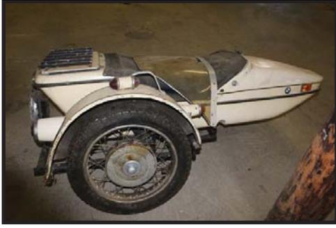
This home-made chassis carries a “hitchhiker” body (believed to be a Californian product) and is set up for a 1955-69 BMW motorcycle, utilizing a BMW wheel and brake assembly. It also uses a BMW “coffee can” taillight. It tracked well when attached to a BMW R60/2.
