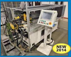
(2) Comco Model TMS-15ND Dual Stack Electric CNC **Tube Benders**
