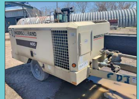
(2) Ingersoll Rand Model VHP-400 Portable Diesel Powered Air Compressors
