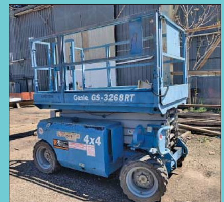
1,000 Lb. Capacity Genie Model GS-3268RT Unleaded Fuel Pneumatic Tire 4X4 Scissor Lift
