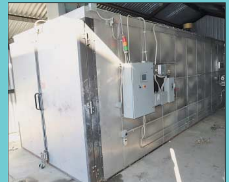
8' x 8' x 20' Spray Tech Systems Model 080820 Natural Gas Drive-In Powder Coat Oven
