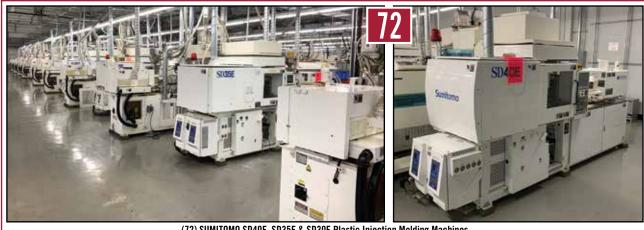
(72) SUMITOMO SD40E, SD35E & SD30E Plastic Injection Molding Machines
