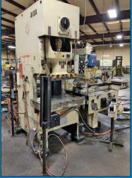
88 Ton Aida Model NC1-80(2) Single Crank Gap Frame Press
