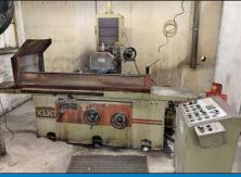
16" x 40" Kent Model KGS410AHD Hydraulic Surface Grinder
