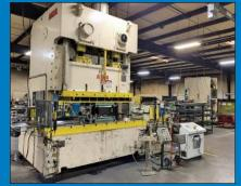
220 Ton Aida Model C2-20(2) Double Crank Gap Frame Press
