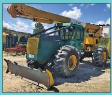
Timberjack Model 240B Cable Std / Shift Articulating 4-Wheel Drive log Skidder
