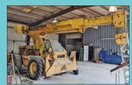
Galion Model 150-A 4-Wheel Drive Rubber Tire Hydraulic Crane
