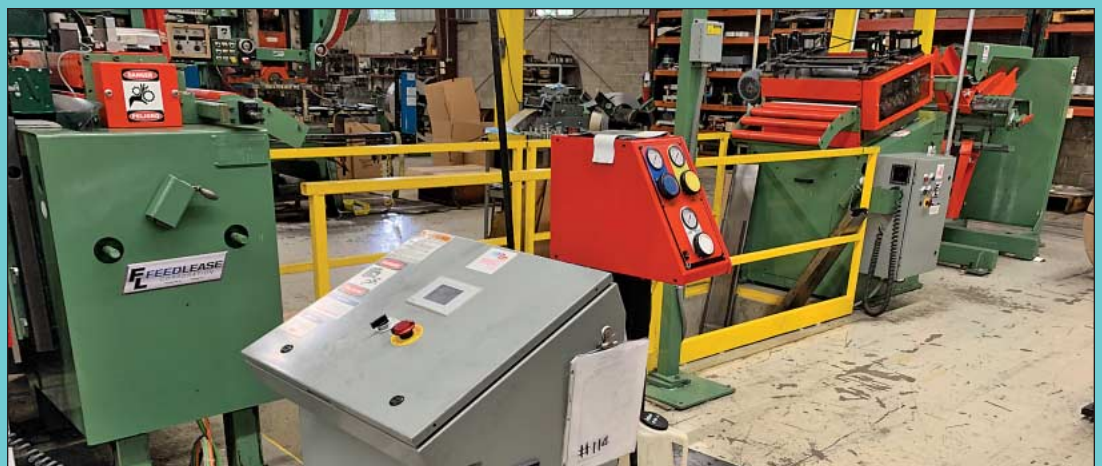
24" wide x 6,000 Lb Feed Lease Press Feed Line Including; 24" w Feed Lease Model PF2.5 24 Servo Feeder, 24" w Feed Lease Model MPS-250-24 Servo Roll Straightener, & 6,000 Lb. Feed Lease Model R-46M-24 Uncoiler
