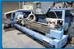
24" x 120" Mazak Model M5 Flat Bed CNC Lathe
