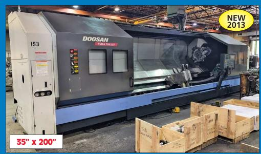
Doosan Puma 700XLY CNC Turning Center, Milling, Y-Axis
