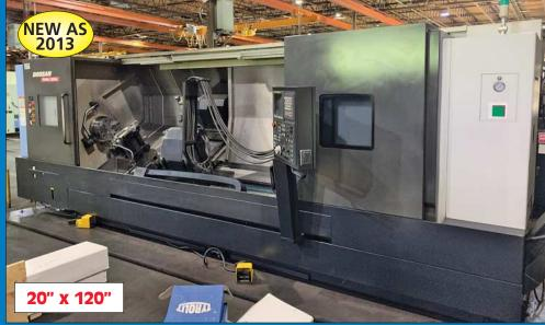
(2) Doosan Puma 3100 CNC Turning Centers, Milling, (1) w/ Y-Axis
