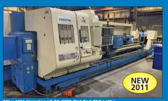
34" x 196" Kingston LC-34x5000 Flat Bed CNC Lathe
