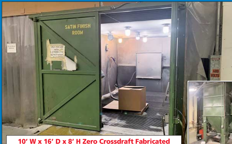
10' W x 16' D x 8' H Zero Crossdraft Fabricated Steel Drive-In Blast Room
