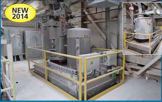
Mixaco HM1200 High Intensity Mixer with HCM4200 Cooler, 440-HP
