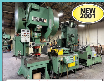
(2) 75 Ton Minster No. 75S OBS Fixed Base Presses
