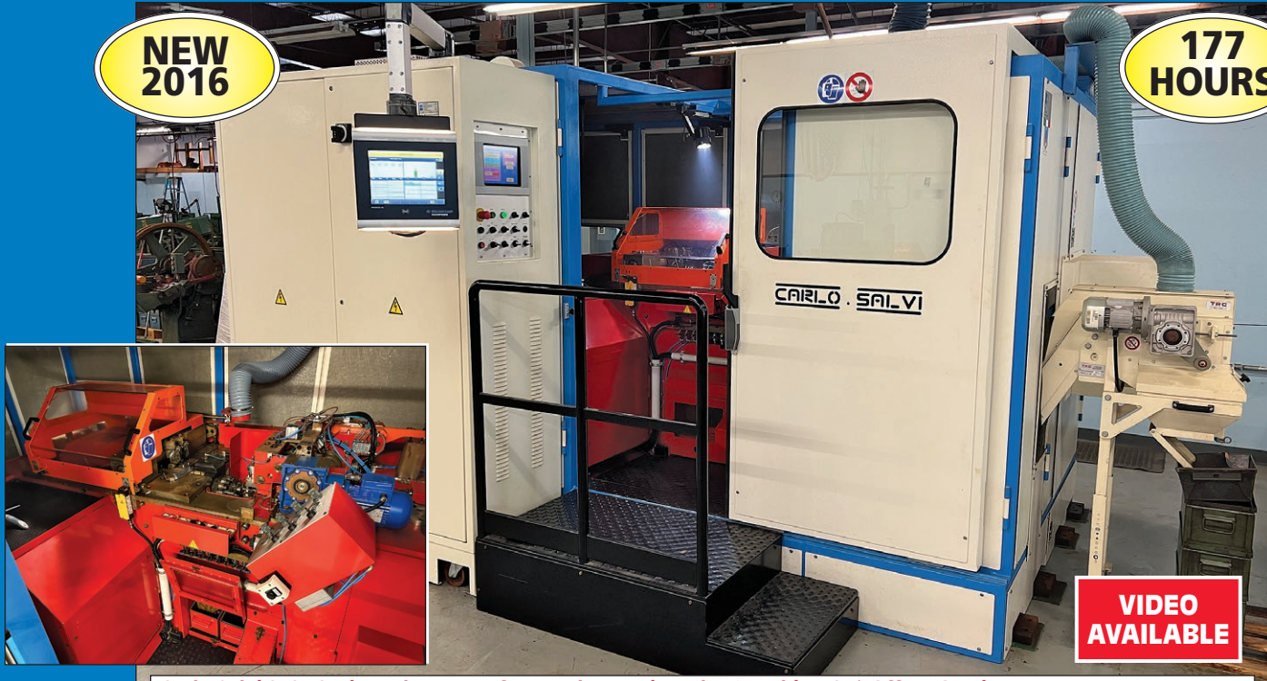
Carlo Salvi 246E 2-Die 4-Blow Transfer Header, Equipped w/ Bushing Cut-Off, PKO, Trim, Semi-Tubular Capable, Linear Feed, Servo Adjustments
