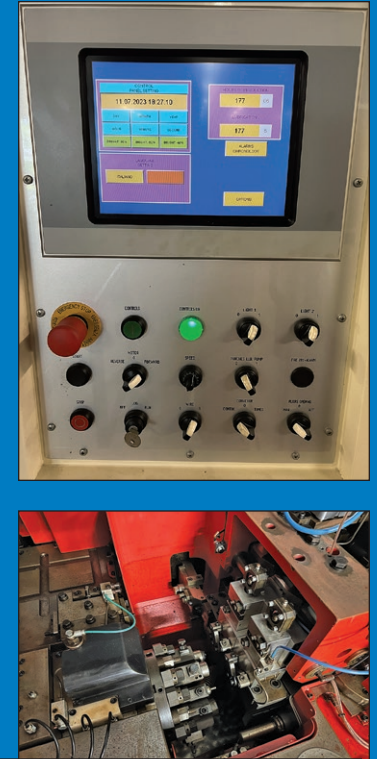
Carlo Salvi 246E 2-Die 4-Blow Transfer Header, Equipped w/ Bushing Cut-Off, PKO, Trim, Semi-Tubular Capable, Linear Feed, Servo Adjustments
