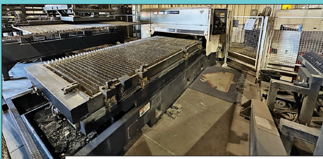
2,500 Watt 5' x 10' Mazak Super Turbo-X510MK II CNC CO2 Laser w/ 10-Shelf FMS
