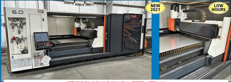
6,000-Watt Mazak Model Optiplex Nexus 3015 Fiber CNC Laser
