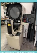
14" MicroVu Model S15 Optical Comparator
