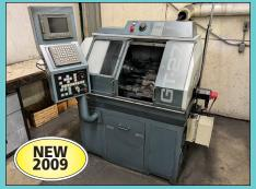
Prodigy / CNC, Inc. Model Fanuc-GT27 CNC Gang Tool Lathe
