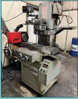
Surface Grinder w/ Haas 4th Axis Indexer / Haas Servo Controller
