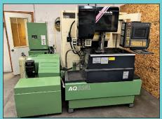
Sodick Model AQ325L Linear Motor CNC Wire EDM
