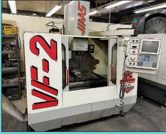
Haas Model VF-2 CNC Vertical Machining Center
