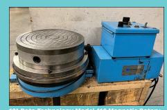
10" Roto Technology Model 410 Magnetic Rotary Table
