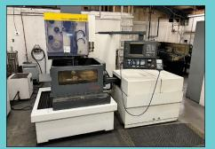
Fanuc Robocut Alpha-1B CNC Wire EDM
