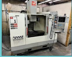
Haas Model VF-1D CNC Vertical Machining Center
