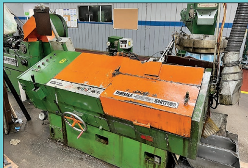
3/8" Tanisaka – Hartford Model 10-400 High Speed Thread Roller
