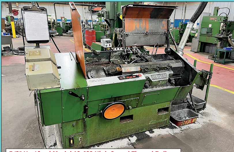
3/8" Hartford Model 10-400 High Speed Thread Roller
