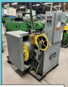
(29) RMG & Fasteners Engineering Wire Drawers 5/16" - 1/8"
