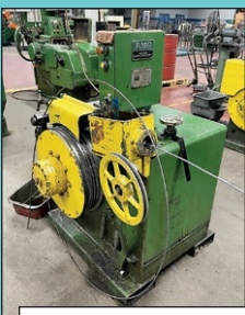
(29) RMG & Fasteners Engineering Wire Drawers 5/16" - 1/8"
