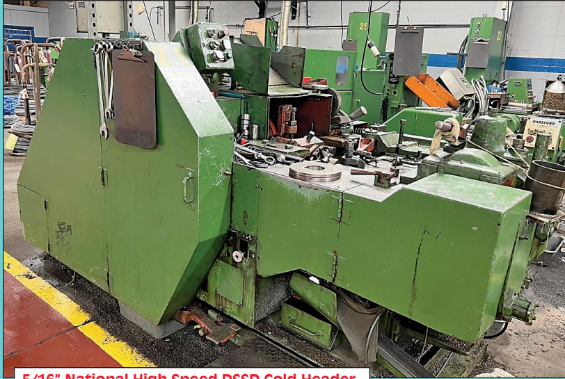
5/16" National High Speed DSSD Cold Header
