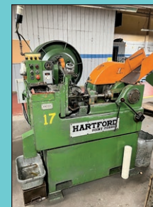
3/8" Hartford Model 6-600 High Speed Pinch Pointers
