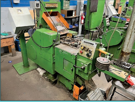
(2) 1/8" Hartford Model 2-450 High Speed DSSD Cold Headers
