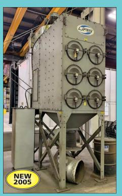
UAS Model SF012-3 Six-Cartridge Dust Collector
