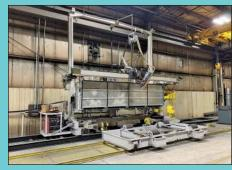
18' Subarc Seam Welding System w/ Lincoln DC-600 Welder, Tank Turning Rolls & 40' Track, 60' Seam Track
