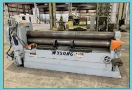
1/4" x 8' Wysong Model F-96 Plate Rolls Hydraulic Plate Bending Rolls
