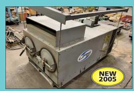
(3) UAS Model SCA Two-Cartridge Fume Collectors
