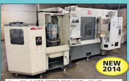
Haas Model EC-400PP CNC HMC with (6) **Station Pallet Changer**
