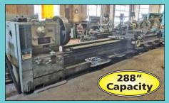
26" X 288" Poreba TPK 80/90A Gap Bed Lathe
