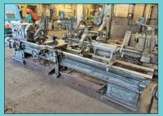
14" X 152" Lehman "Hydrotral" Engine Lathe
