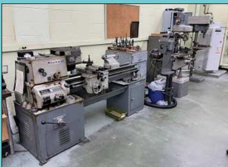
Toolroom Machinery including Lathe, Mill, Drill, and More
