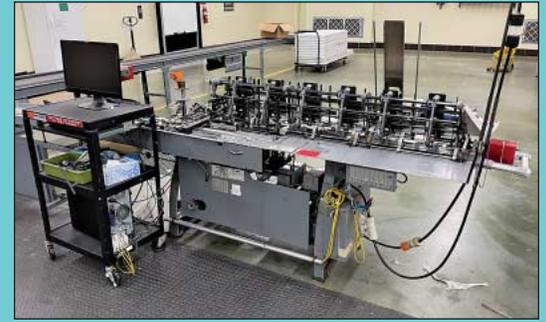
(2) Bell & Howell Model A340-6 Six-Pocket Inserters w/ Stream Feeders
