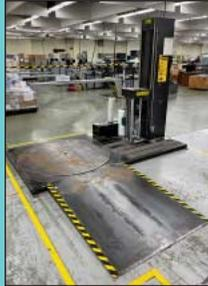
60" IPM Model LPUTS30F Rotary Stretch Wrapper w/ Ramp
