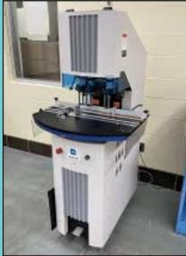
Baum Model D3 Three-Spindle Paper Drill
