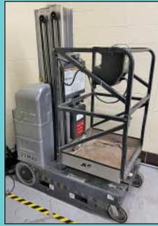
JLG Model 30MVL Electric Portable Man Lift
