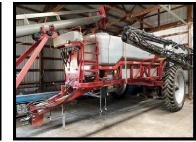
RedBall 580 Sprayer, Approx 1600 Gal Tank, Adj Axle, 6 Section 90'Boom, Rinse & Fresh Tank, Triple Nozzles, 380/90R46 Singles
