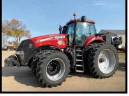
2013 Case IH 315 Magnum MFWD Tractor, 23 Speed PS, Luxury Suspension Cab, Leather, AutoGuidance, Front Axle Susp, 4 SCV, Cat 4N/3 3Pt, QH, 1-3/4" 1000 PTO, Hi-Cap Hyd Pump, Performance Cluster, Positive Response Seat, Int Seat, Power Mirrors, HID Lights, Front Fenders, BlueTooth Radio, RH Wiper, (6) Suitcase Weights, Pro 700 RTK, 480/80R50 Rear Duals, 420/85R34 Front Duals, 1765 Hours Showing, SN-ZDRD06134
