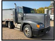
1996 Freightliner FLD 120 Day Cab Semi Tractor, 10 Spd E&F Trans, 561,263 Miles, N14 Cummins Plus, LoPro 22.5 on Alum Front, Steel Rear, Hub Pilot, Sliding 5th Wheel, Dual Alum Tanks, VIN: 1FUYDCYB7TP779075
