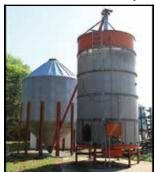
Butler Kan-Sun Grain Dryer, Stainless Screens, 440V 3 Ph, (2) 10 Hp Motors, Model- 10-21-210, SN- SC100873 Stormor Grain Bin, Approx 25000 Bu, 9.5 Ring, 36' Dia, (2) Roof Vents
