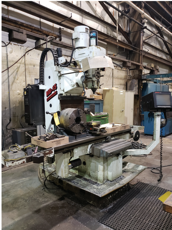
Fryer MB-15, SN 905 0909547, 15-1/2" x 67" table, 30 taper, Anilam 1100M controls, travels - X-50, Y-22, 24" under spindle
