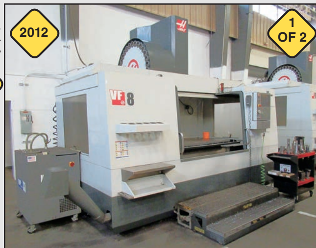
Haas VF8/50 4-Axis Vertical Machining Center with High Pressure Coolant
