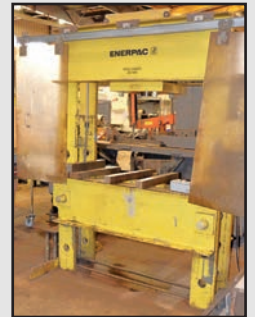
150-Ton Enerpac H-Frame Hydraulic Press with Sliding Head
