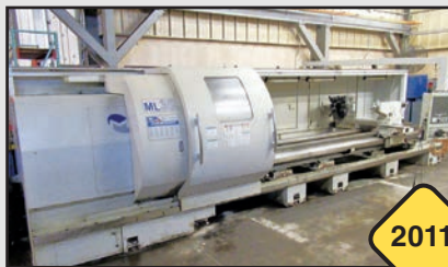
36" x 200" Milltronics ML35 CNC Lathe with Milling
