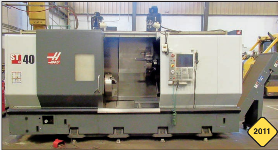
Haas ST-40 "Big Bore" CNC Turning Center with Live Milling
