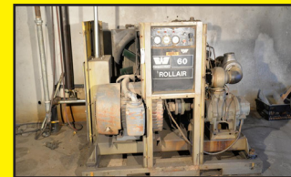
WORTHINGTON ROLLAIR 60 AIR COMPRESSOR, 100 HP, CHIMLEY ELEC. INDUCTION MOTOR, MD. 5K365BK174, 75 HP, 640 VOLTS, 3560 RPM, AMERITHON FAN MOTOR, 2HP
