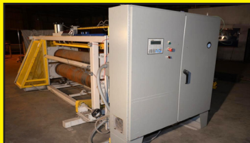
LAMINATOR MACHINE MADE AT THIS FACILITY BY PARENT COMPANY. LAMINATES BACK OF CARPET PADDING - HEATING COIL NEEDS REPAIR
