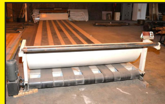
J BOX CONVEYOR - 28 FT. ELECTRIC MOTOR
