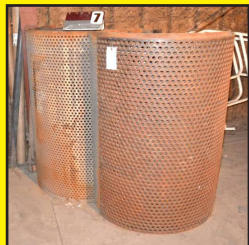
(7) STEEL OVAL SCREENS 32" DIA. - 5/8" STAGGERED HOLE PATTERN
