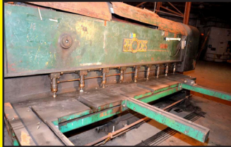
RHODES SHEAR 12' X 1/4" CAPACITY - WORKS - RHODES PATENT QUOTE NO. 10001
