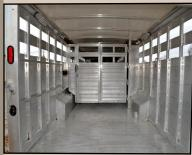
ADJUSTABLE HT STEM (GN STD) ~ TAPERED SIDES 2/18" R **CORNERS NOSE PROFILE ~ GATES: REAR OPENING SWING** TYPE W/ SLIDING GATE ~ HEAVY DUTY STEEL CAM LOCK ~ SEALED ACCESS GATE 34" W/ BLK LATCH ~ 16" TALL **FOLD-DOWN GOOSENECK GATE ~ TRAVELING CENTER** SWINGING TYPE GATE W/ SLIDER - TRACK LINK 10 FT. LONG ~ SIDE RAMP: FULL HEIGHT UP TO 48" WIDE, SEALED W/ **BLK LATCHES ~**
