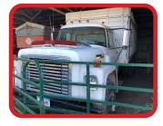
**GRAIN TRUCK** 1974 IH Loadstar, 392 rebuilt, 18'Obeco steel box. 5-4 transmission, 18 ft, Twin Screw. Shedded, road ready, 200,000 miles
