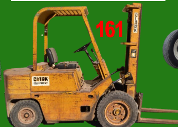
Clark pneumatic forklift 5,500 lb, gas, 48" forks, 5,500# lift capacity
