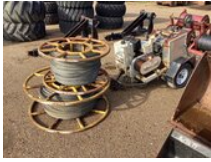
#2905 • CONDUX ROPE PULLER 5,600LBS MAX PULL CAPACITY, 2 ROLLS OF ROPE, DIESEL ENGINE, TRAILER MTD - NO TITLE ON TRAILER
