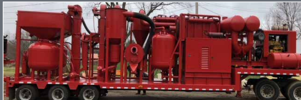
ARS ARIES/VAC BLAST RECYCLING MACHINE WITH 60KW GENERATOR AND JOHN DEERE DIESEL ENGINE
