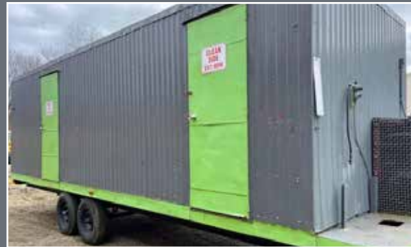
ACSI DECONTAMINATION TRAILER EQUIPPED WITH STEPS AND SHOWERS AND HOT WATER HEATER
