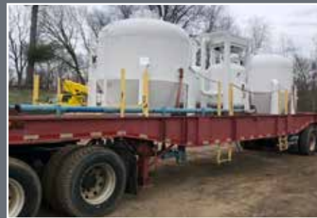
ACSI DECONTAMINATION TRAILER EQUIPPED WITH STEPS AND SHOWERS AND HOT WATER HEATER
