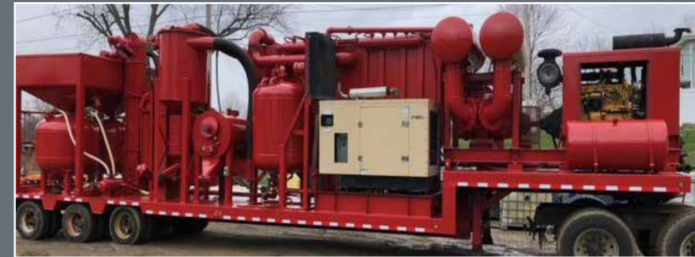
ARS ARIES/VAC BLAST RECYCLING MACHINE WITH 60KW GENERATOR AND JOHN DEERE DIESEL ENGINE
