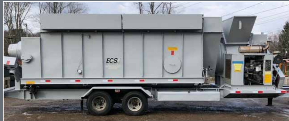
ECS P40 DUST COLLECTOR 40,000CFM POWERED BY A 5.9 CUMMINS ENGINE/FUNCTIONAL UNIT
