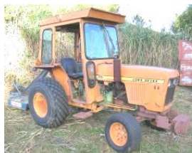
John Deere 850 Tractor, 3 Cyl Dsl W/Cab, 2wd, Rr 13-6-16 Turf Tires W/3 Pt 4' King Cutter Brush Hog,
