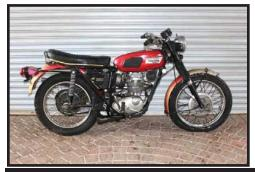
•250 CC single-cylinder•Square tank•Stock exhaust with high-pipe
