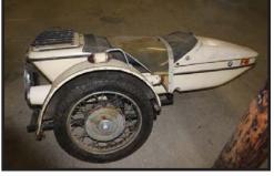
This home-made chassis carries a "hitchhiker" body (believed to be a Californian product) and is set up for a 1955-69 BMW motorcycle, utilizing a BMW wheel and brake assembly. It also uses a BMW "coffee can" taillight. It tracked well when attached to a BMW R60/2.
